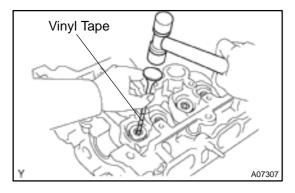
(d) Using a plastic–faced hammer and the valve stem (not in use) tip wound with vinyl tape, lightly tap the valve stem tip to ensure a proper fit.
