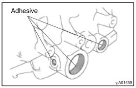
(b) Apply adhesive to the water hose union hole of the cylinder head
