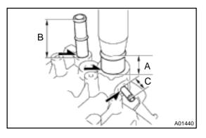
(c) Using a press, press in a new water hose union until it is protruding from the cylinder head.
