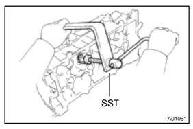
(c) Using SST, compress the valve spring and place the 2 keepers around the valve stem.
