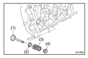
(b) Install the valve (1), spring (2), valve spring (3) and spring retainer (4).
